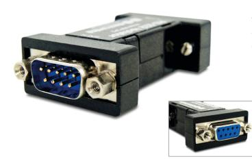
The RS232 Isolator STD 2.5KV B 9Pin optically isolates both the RS-232 transmit and receive lines. The isolator has a DB9S female connector on the DTE side and a DB9P male connector on the DCE side. Typical DTE devices include PCs, terminals, and printers. Typical DCE devices include modems and mul-
