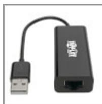
Connects your USB-enabled computer or laptop to a 10/100 Mbps Ethernet network without installing an internal Ethernet card.
